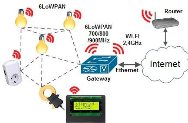
Fig. 1. Smart building system with energy monitoring and smart lightning system
