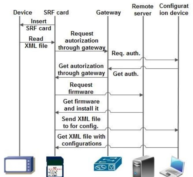
Fig. 9. New device configuration process
