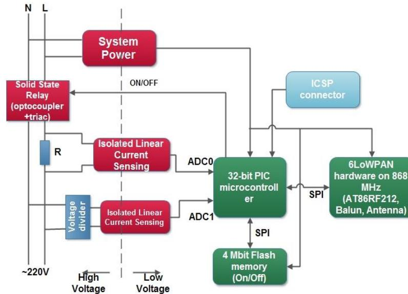
Fig. 2. Device level energy consumption measurement device block schematic
