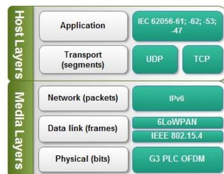
Fig. 6. ISO/OSI model for G3 protocol having IPv6, 802.15.4 and 6LoWPAN support layers
