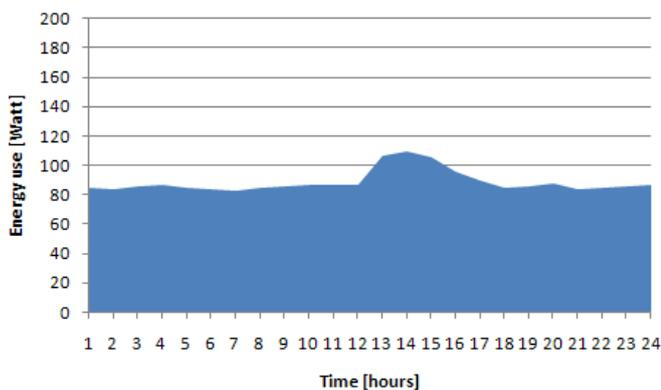
Fig. 10. Device level energy use monitoring for a refrigerator
