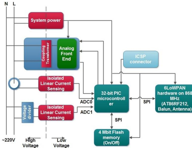
Fig. 4. Household level energy consumption measurement device block schematic
