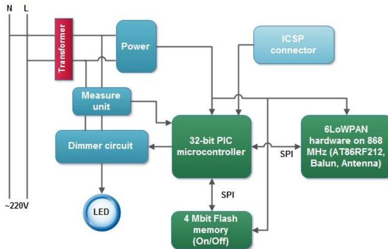
Fig. 7. LightBox block schematic
