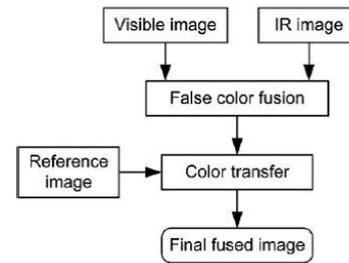
Fig 1 Schematic Diagram of One Color Contrast Enhanced Image Fusion
