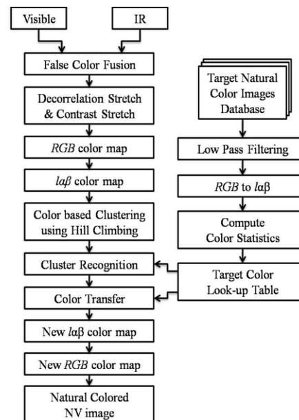
Fig 5 Efficient Color Transfer Algorithm
