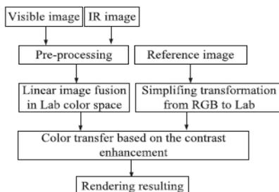
Fig 4 Fast Color Contrast Enhancement Method
