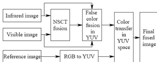
Fig 3 Adaptive Color Fusion Method
