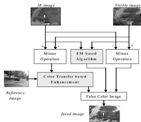
Fig 2 Color Fusion Based on EM Algorithm method
