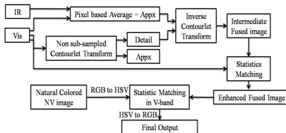
Fig 6 Block diagram of the Image Fusion Algorithm
