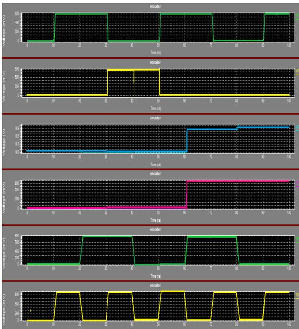
Figure 4(b) Waveforms of CMOS dual encoder
