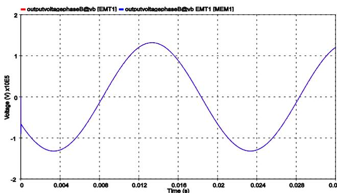
Fig 7 Transient voltage wave from during closing operation of CB for 10mts length in a B-phase of 132kv GIS
