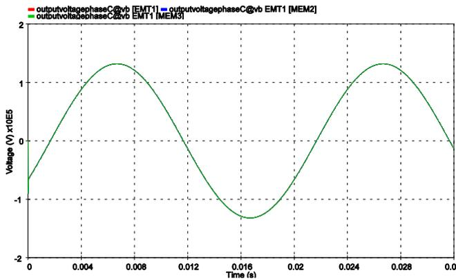
Fig.10 Transient voltage waveform during second re-strikes for 10mts length in a B-phase of 132kv GIS
