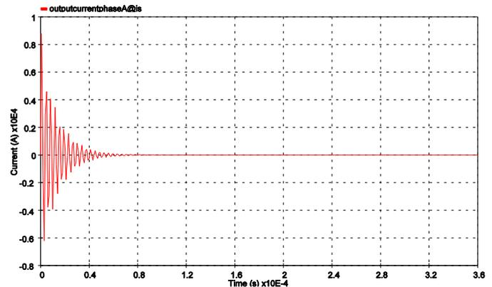
Fig. 4 Current waveform during closing operation of CB for 10mts length in a A-phase of 132kv GIS
