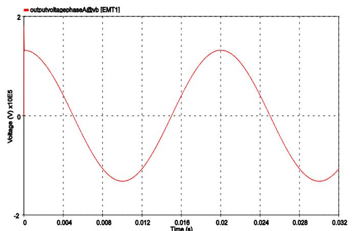
Fig.9 Transient voltage waveform during second re-strikes for 10mts length in a A-phase of 132kv GIS
