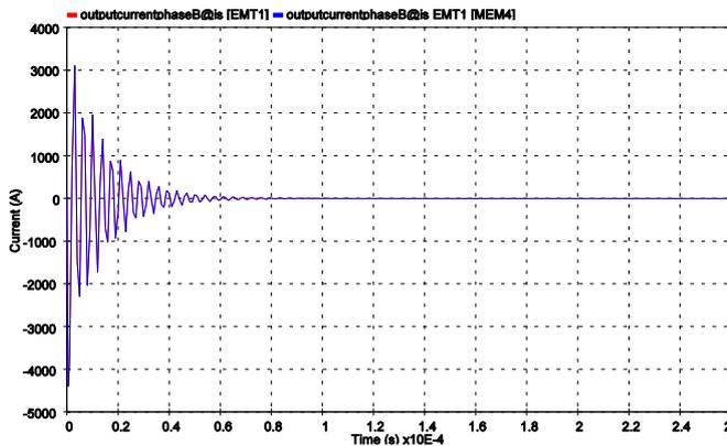
Fig. 5 Current waveform during closing operation of CB for 10mts length in a B-phase of 132kv GIS
