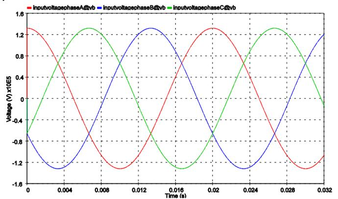
Fig. 8 Transient voltage waveform during opening operation of CB for 10mts length in a 3-phase to 2-phase(C Phase Earthed) of 132kv GIS
