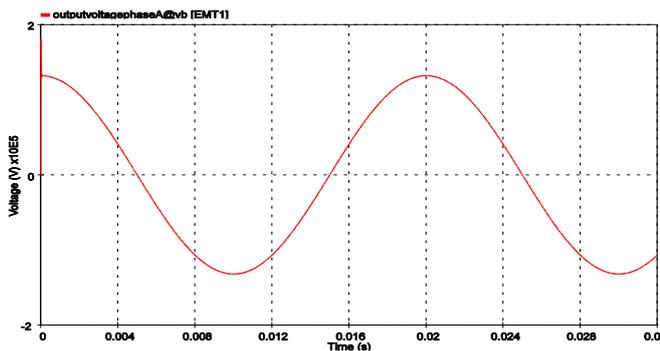
Fig 6 Transient voltage wave from during closing operation of CB for 10mts length in a A-phase of 132kv GIS
