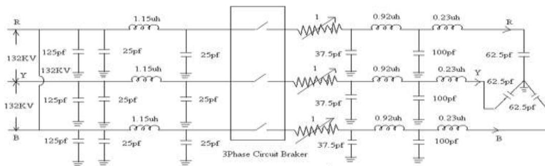
Fig. 2. Equivalent circuit for 10mtrs. Length in a 3 -phase to 2-phase of a 132kv GIS
