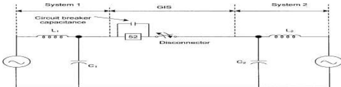
Fig 1.A disconnecter in GIS, interconnecting two systems, possible switching in phase opposition
