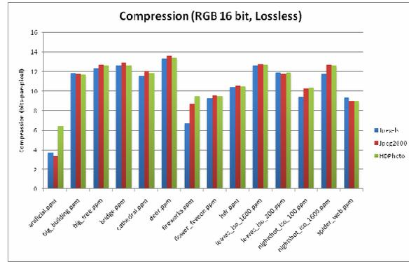
Fig.10: Compression on 16 bit RGB image.
