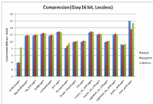
Fig.9: Compression on 16 bit gray scale image.
