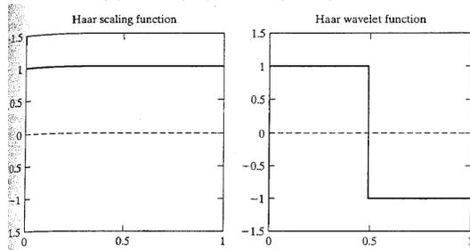
Fig.8: An Example of Haar scaling function.
