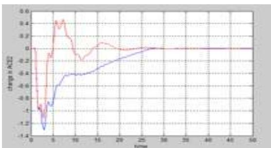
Figure 15: Area control error of area 2 by both PI and fuzzy logic controller
