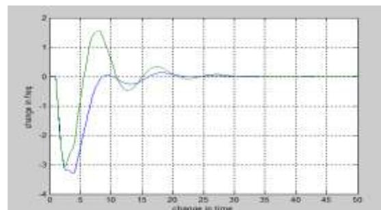
Figure 16: Frequency Response comparison using Conventional PI and FLC controller in area 1
