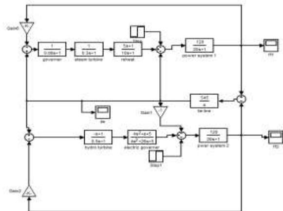
Figure 7: Interconnected systems without any controller
