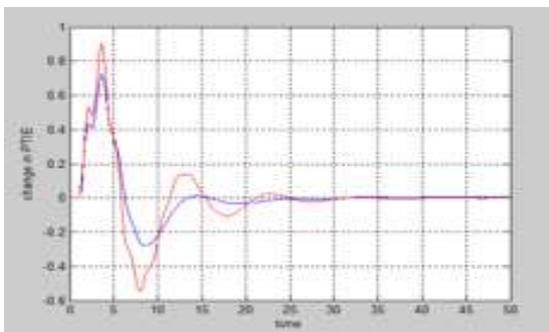
Figure 14: Tie line deviation by both PI and fuzzy logic controller
