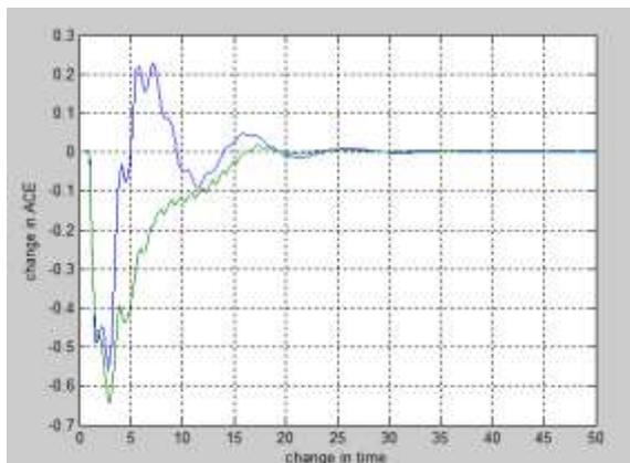
Figure 19: ACE Response comparison using Conventional PI and FLC controller in area 2
