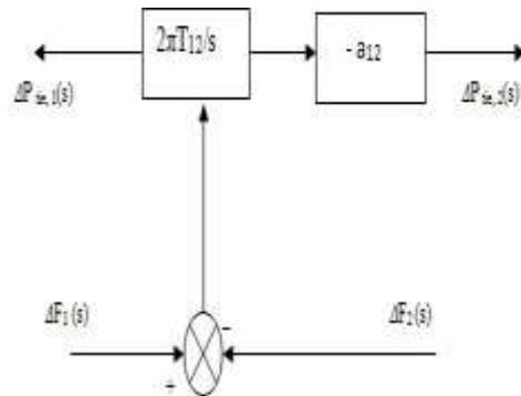
Figure 3: Transfer function of tie line power
