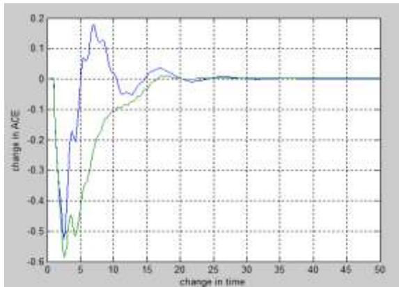
Figure 18: ACE Response comparison using Conventional PI and FLC controller in area 1
