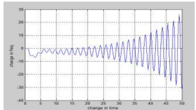
Figure 11: Frequency Response without using controller in area 2
