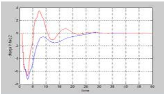
Figure 13: Frequency deviation of area 2 by both PI and fuzzy logic controller
