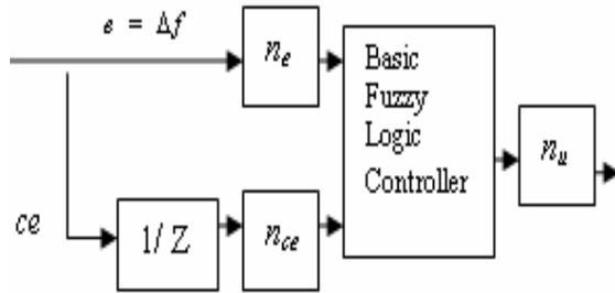
Figure 5: Block diagram of a fuzzy logic controller.
