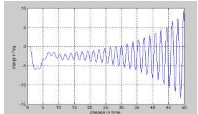
Figure 10: Frequency Response with out using controller in area 1
