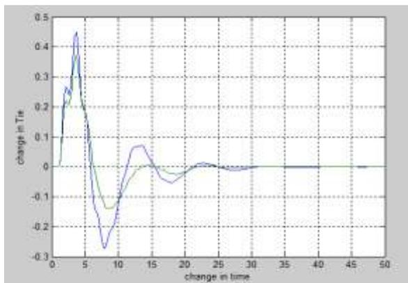
Figure 20: Tie Line Response comparison using Conventional PI and FLC controller.
