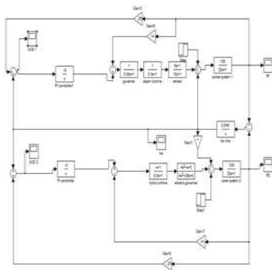
Figure 9: FLC using conventional PI controller
