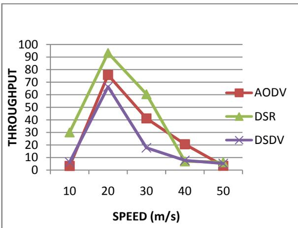
Figure 5. Throughput vs. Speed
