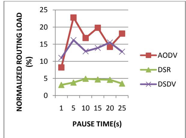
Figure 13. Normalized Routing Load vs. Pause Time
