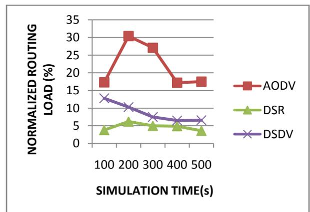
Figure 15. Normalized routing Load vs. Simulation Time
