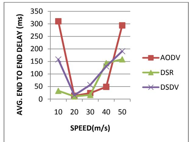
Figure 8. Avg. E2E Delay vs. Speed
