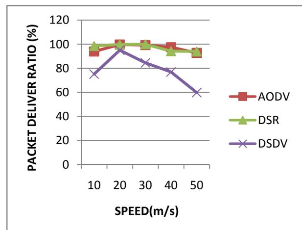
Figure 2. Packet Delivery Ratio vs. Speed
