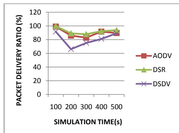
Figure 3. Packet Delivery Ratio vs. Simulation Time
