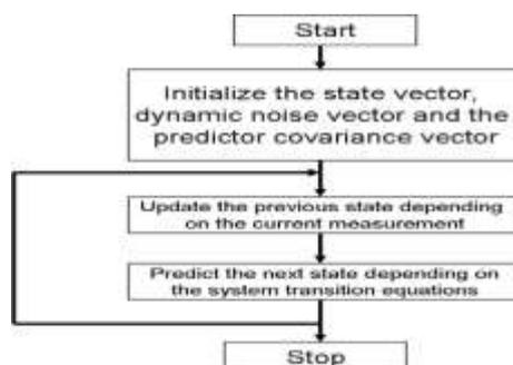
Fig 6:Algorithm for Kalman Filter
