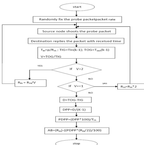
Fig.3 Flow chart of working proposed system
