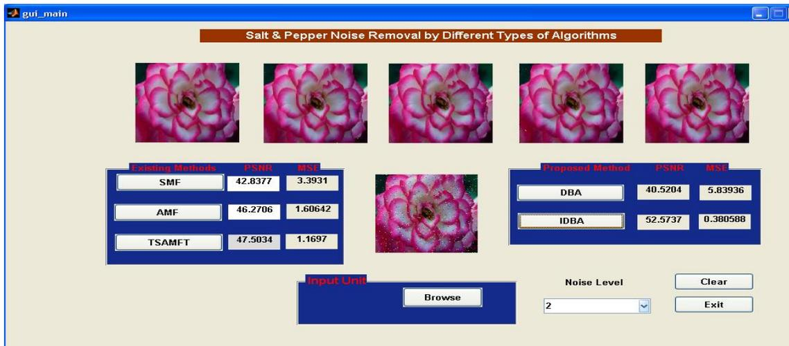
Figure4. Color image Restoration with SMF,AMF,TSAMF,DBA,DBUTMF
