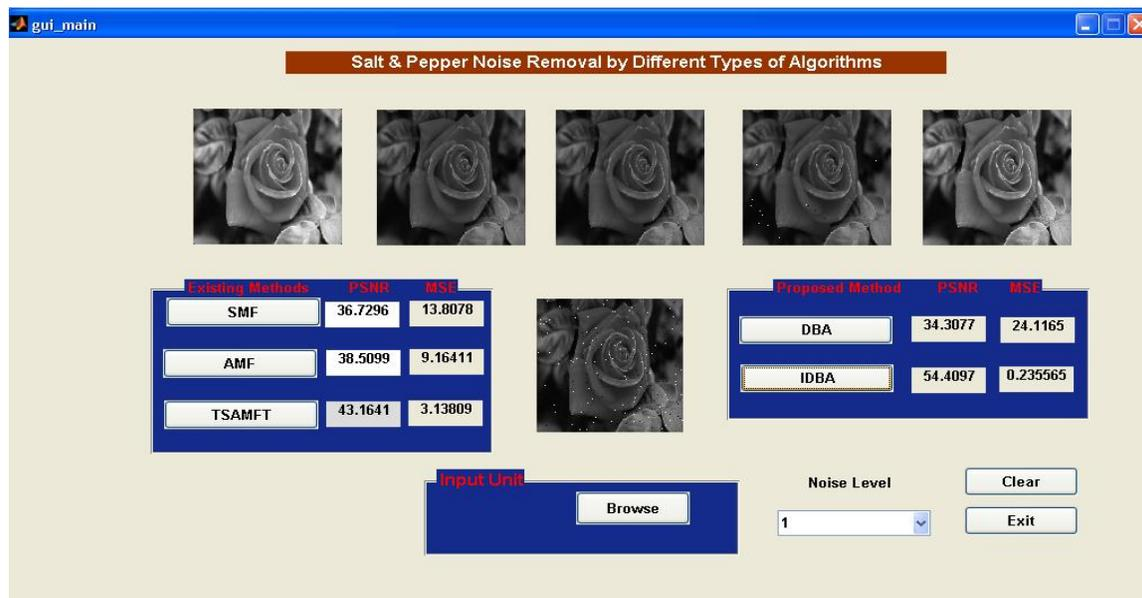
Figure2: Grayscale image Restoration with SMF,AMF,TSAMF,DBA,DBUTMF
