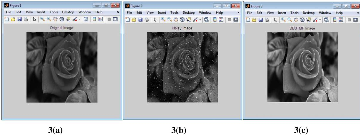
Figure3.: The proposed DBUTMF application for gray scale images 3(a).Original image 3(b).Noisy image, 3(c).Restoration with the proposed MDBUTMF.
