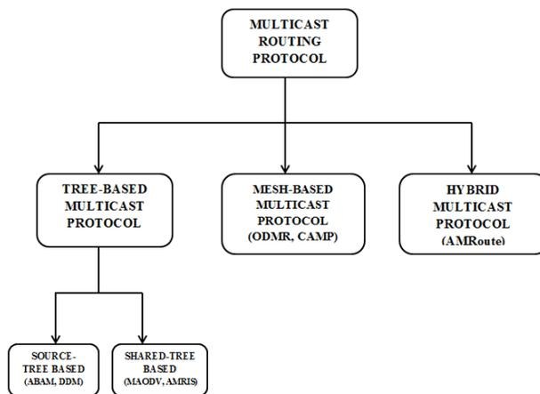
**Fig1: Multicast routing protocols**
