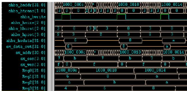
Figure 13. Write with zero wait state to RAM
