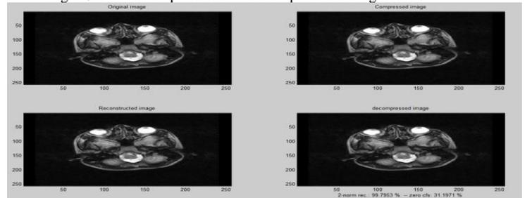
Fig. 1.10 2-level compression and decompression using Bior1.3
