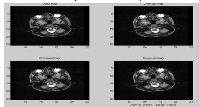
Fig 1.1.Haar first level compression and decompression
