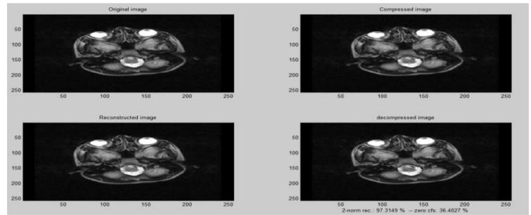
Fig. 1.8 level-4 compression and decompression using db2
