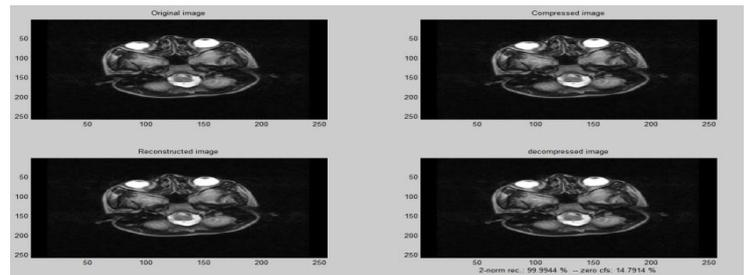
Fig. 1.9 1-level compression and decompression using Bior1.3
