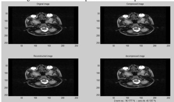
Fig. 1.4 Haar 4-level compression and decompression
