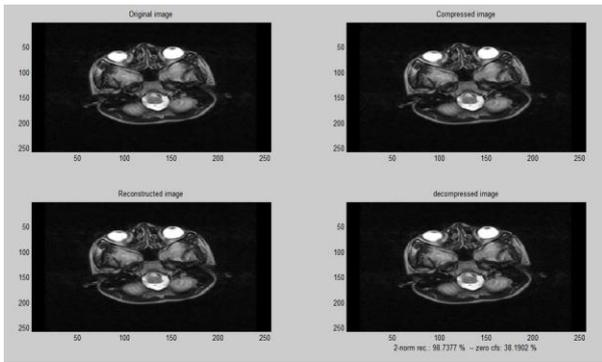
Fig 1.3. Haar 3-level compression and decompression
