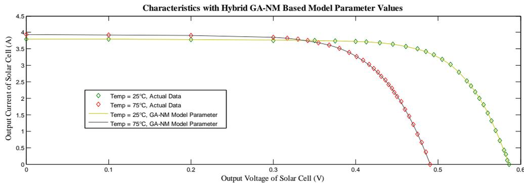
Fig 3: I-V Characteristics Using Actual Data and GA-NM Estimated Results
