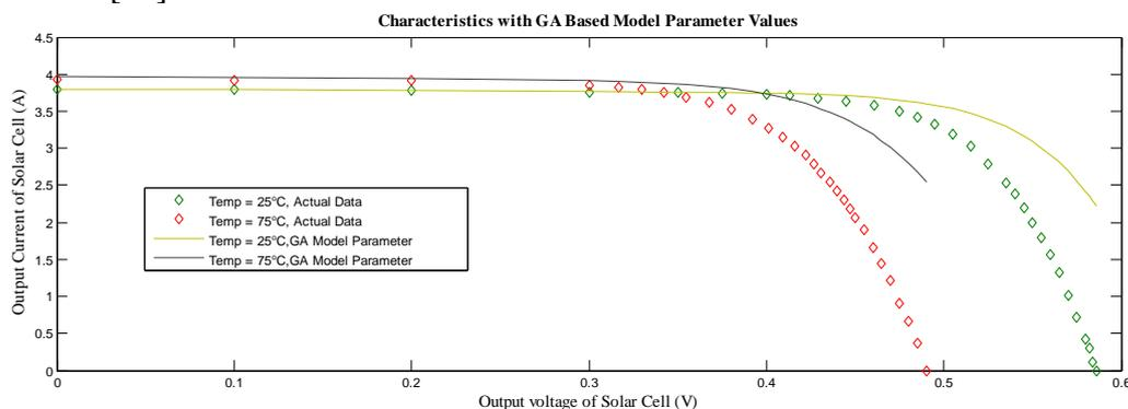
Fig 2: I-V Characteristics Using Actual Data and GA Estimated Results
