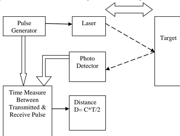
Fig. (a) Distance Measurement with Laser ( $C$ = velocity of light)
