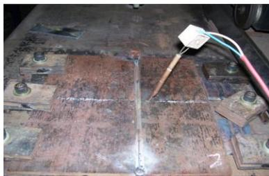
**Figure 3. Thermocouple setup**
