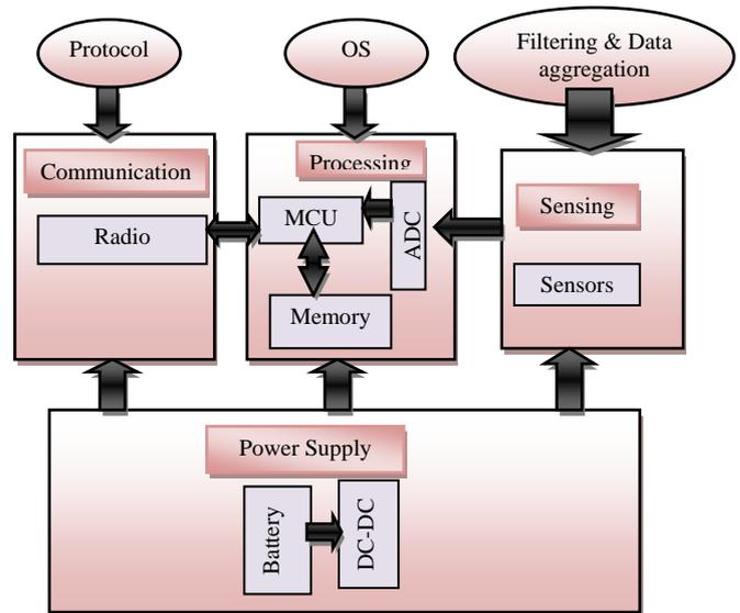
**Figure 1.2 Sensor node architectures**
