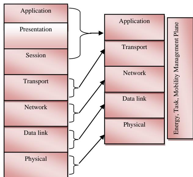
**Figure 1.3 Protocol stack for Wireless Sensor Networks**
