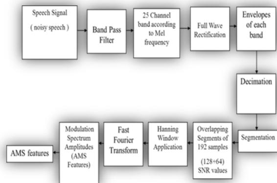
Fig 1. Block Diagram of Feature Extraction
