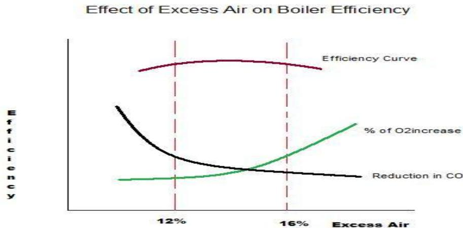
**Fig:-Excess air on boiler efficiency**
