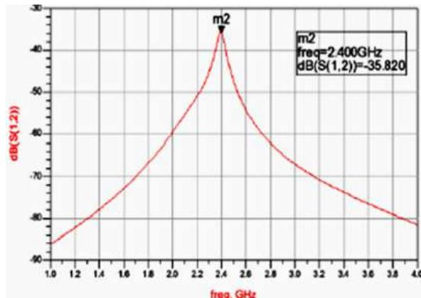
Figure 13: Reverse Isolation of more than -35 dB.
