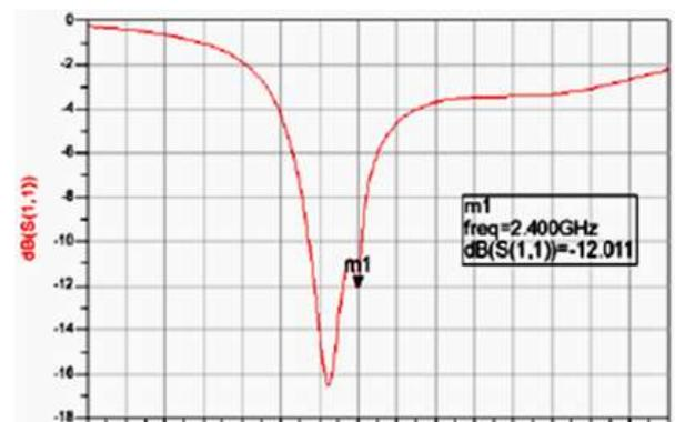
Figure 11: Reverse isolation of LNA (More than -12 dB)
