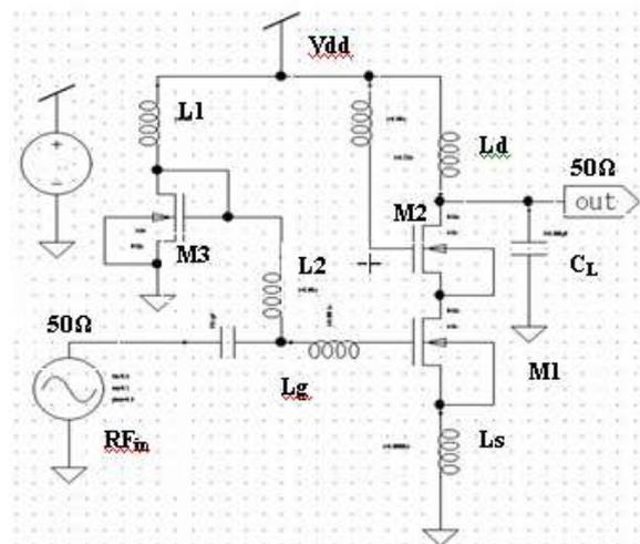
Figure 2: Proposed LNA schematic design with inductors replacing all resistive components for reduction of thermal noise .
