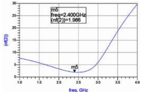
Figure 10: Noise figure of the LNA (Minimum Noise Figure is 1.986 dB at 2.4 GHz)
