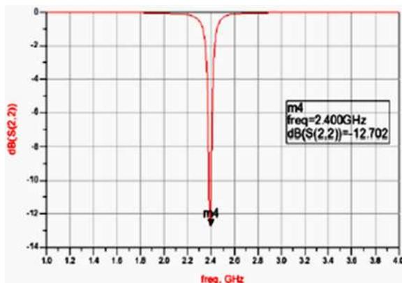
Figure 14: S22 Output Reflection Coefficient -13 dB
