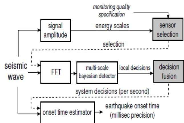
Fig.5 System Architecture White blocks are the components at a sensor; shadowed blocks are the components at the base station; solid line represents data flow; dotted line represents control flow
