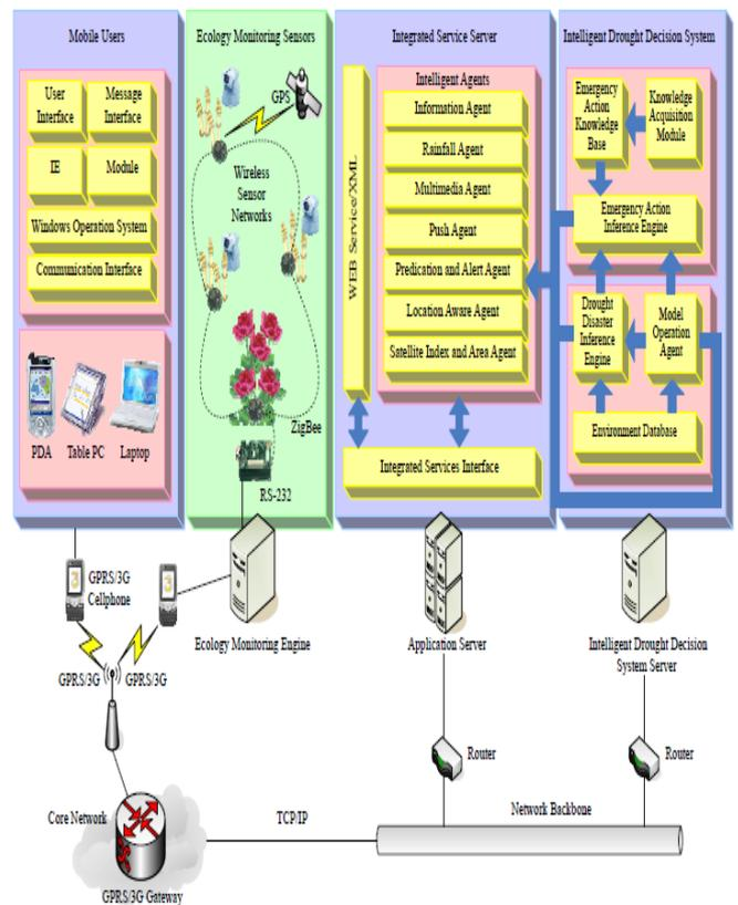
Fig.7 Drought forecast and alert system and network architecture
