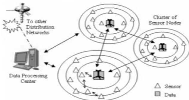
Fig.2 Data collection and aggregation in wireless sensor network
