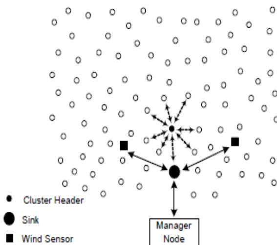
Fig.4 A wireless sensor network for real-time forest fire detection
