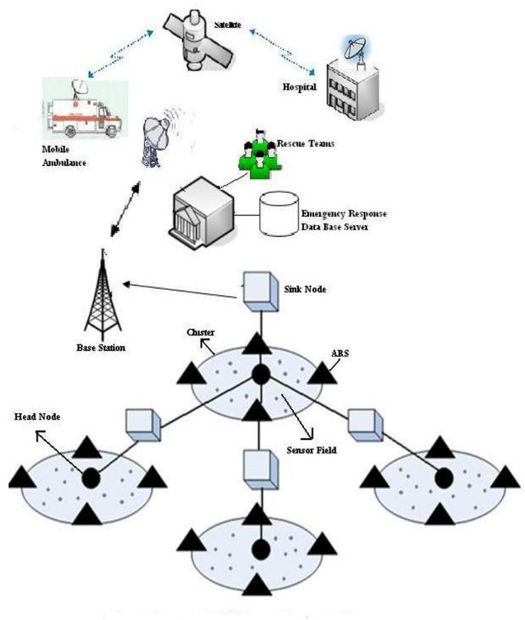
Fig.1. Wireless Sensor Network Architecture for disaster survivor detection
