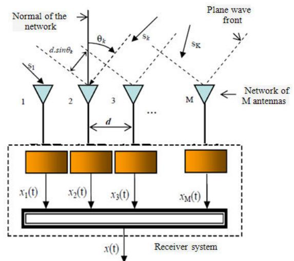
Fig.1 Network of M antennas and receiver system with K incident signals.
