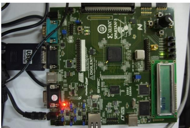
Figure 7 : Spartan 3AN Starter Kit connected to a D-Link Switch for testing the logic of developed distributed embedded system
