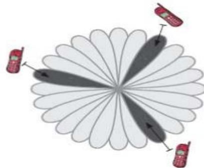
Fig .3.3 Working of Switched beam arrays
