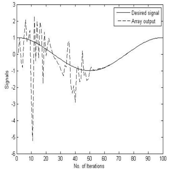
Fig 4.5 Convergence of LMS algorithm
