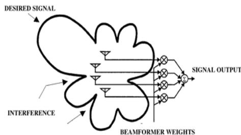
Fig 3.4 Adaptive beamforming
