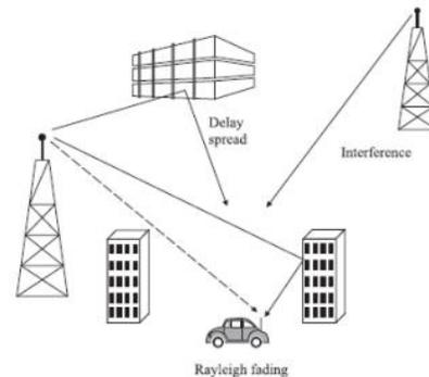
**Fig 3.1 Wireless communication impairments that smart antennas have to combat**
