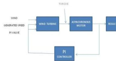
Wind turbine scheme with pi controller
