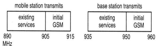
Fig: GSM Frequency Band
