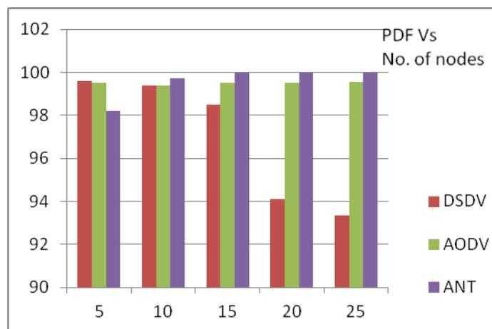
Fig.2 Comparison of Packet Delivery Fraction (PDF)
