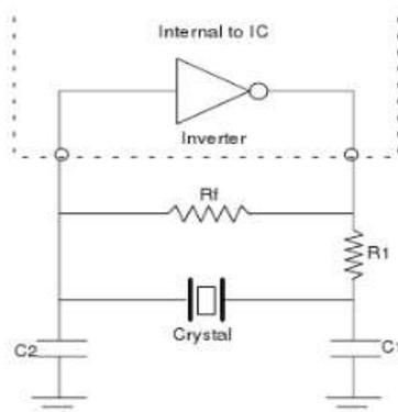
Figure1: Crystal Oscillator Circuit.
