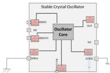
Figure2: On-Chip Crystal Oscillator with ESD protection
