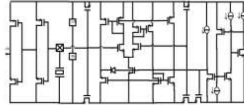
Figure3: Complete Schematic Diagram Of The Crystal Oscillator
