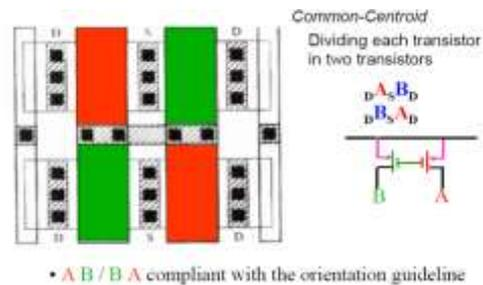
Figure6: Common-Centroid Technique
