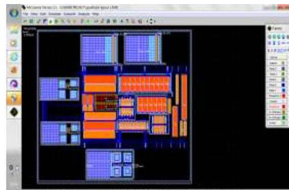
Figure4: Layout Diagram Of The Crystal Oscillator Circuit
