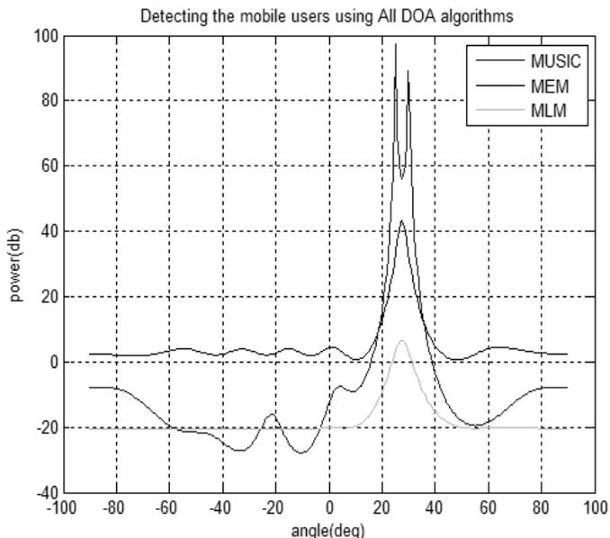
**Fig. 7. Comparisons of MLM, MEM and MUSIC Method for closely spaced sources with less antenna elements.**
