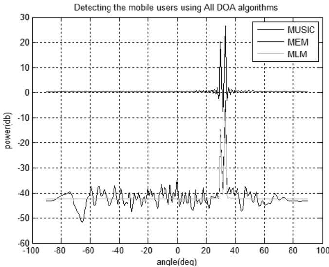
**Fig. 9. Comparisons of MLM, MEM and MUSIC Method for closely spaced sources with more antenna elements.**
