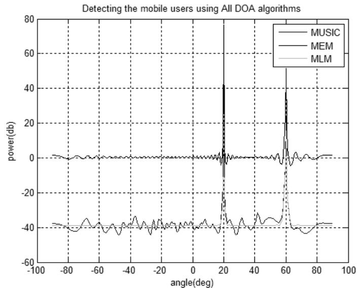
**Fig. 8. Comparisons of MLM, MEM and MUSIC Method for widely spaced sources with less antenna elements.**
