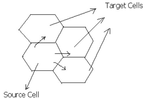
Fig4. Target cell based handover.
