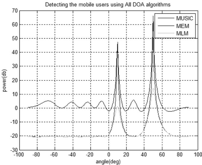
**Fig. 6. Comparisons of MLM, MEM and MUSIC Method for widely spaced sources with less antenna elements.**
