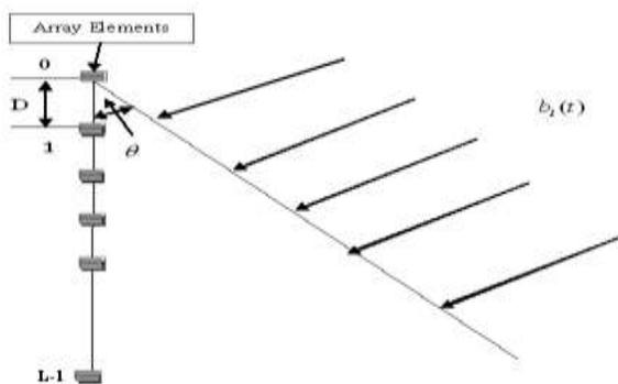
Fig. 2. Uniform Linear Array.
