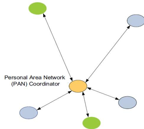
Fig.3 Zigbee Network
