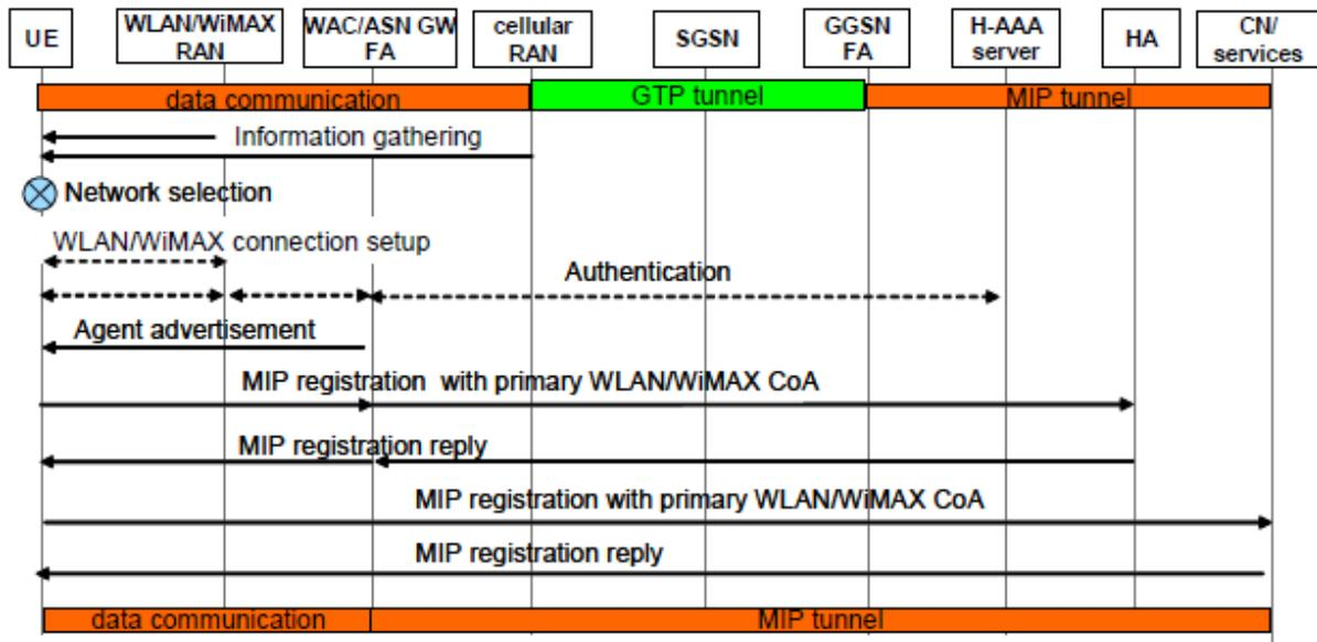
Fig 2 .Handover from 3GPP to WLAN/WiMax
