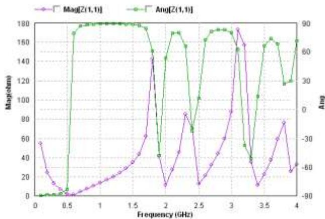
Figure 7. Z parameters (Z11) Vs frequency plot of RMA on IE3D
