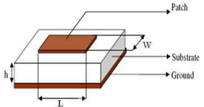
Figure 1. Rectangular Microstrip Patch Antenna
