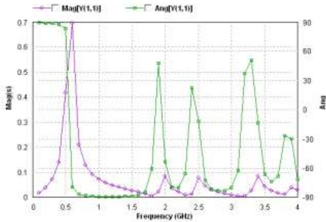
Figure 6. Y parameters (Y11) Vs frequency plot of RMA on IE3D
