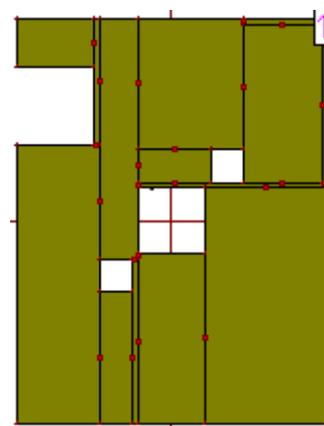
Figure 2. Geometry of notched square slot loaded microstrip antenna
