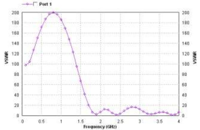
Figure 9 . VSWR parameters Vs frequency plot of RMA on IE3D
