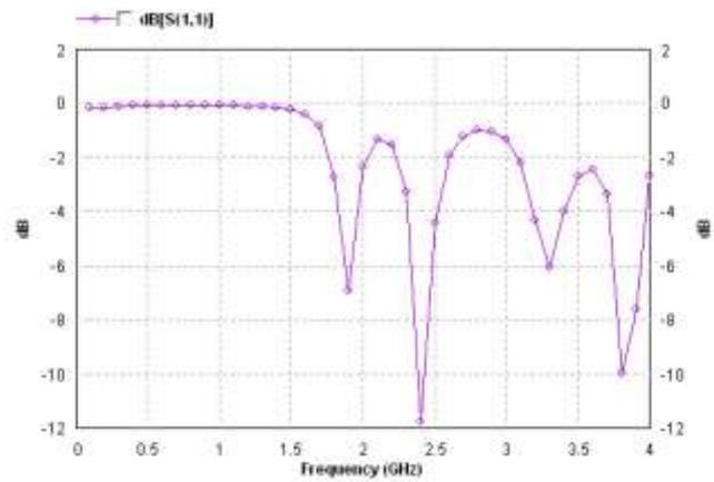
Figure 4. . Return loss(S11) Vs frequency plot of RMA on IE3D
