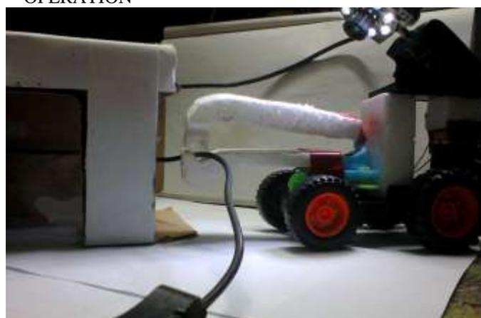
FIGURE 11 : ROBOT IN ACTION WITH HOLDING A CABLE , CLEARING IT FROM A NARROW CHANEL
