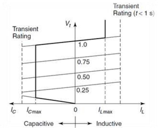
Fig.1. the V-I characteristic of the STATCOM [3].
