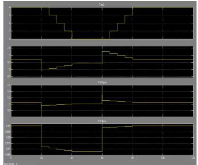
**Fig.5. Coordination of STATCOM and ULTC without fixed capacitor**
