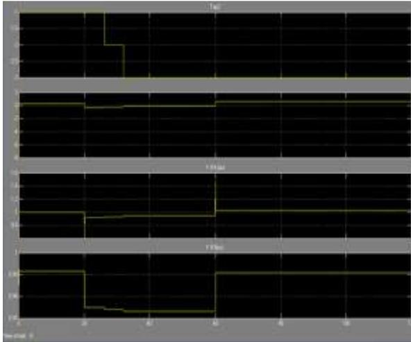
**Fig.7. Operation of STATCOM and ULTC without coordination (with fixed capacitor)**
