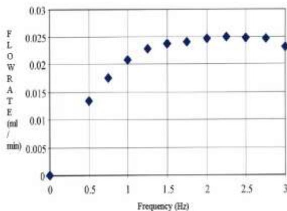
FIG-7 Simulation results of Cumulative Flow rate as a function of the frequency
