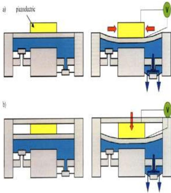
**FIG-1.a)** piezoelectric actuator in the lateral-strain configuration. b) Piezoelectric actuator in the axial strain configuration.
