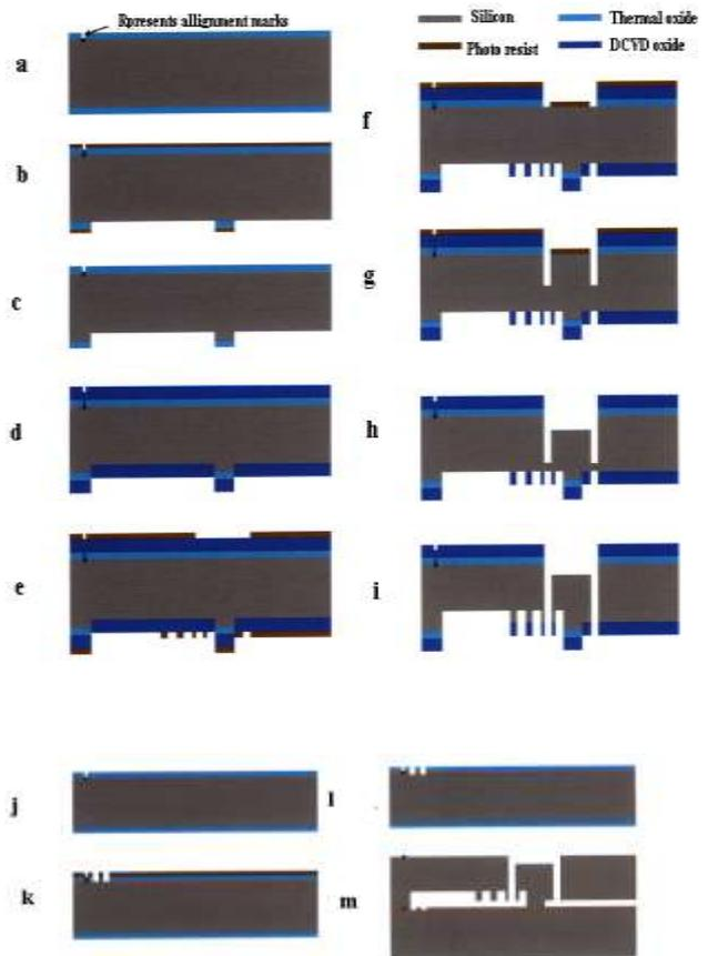
**FIG- 2.**(a-m) Different CAD Layout of the micropump Layer
