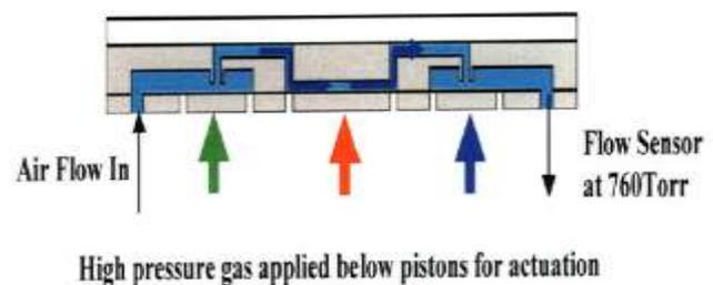
pressure the pistons should actuate shut and the output flow should drop to zero
