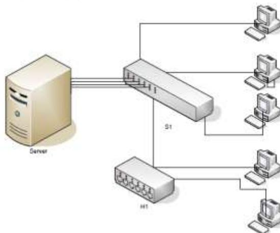
Fig 2 A Sample Model of switch-to-server connection
