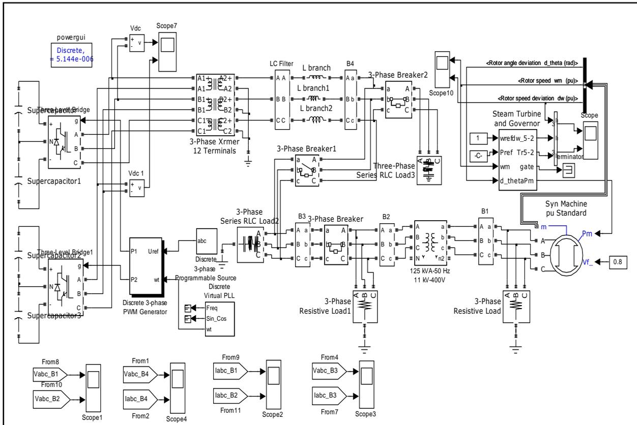
Fig. A. Simulation model based on super capacitor based energy storage system
