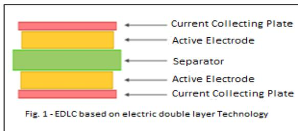
They offer high power densities and provide significant energy storage capacities. It stores the energy in the double layer formed near the carbon electrode surface.
