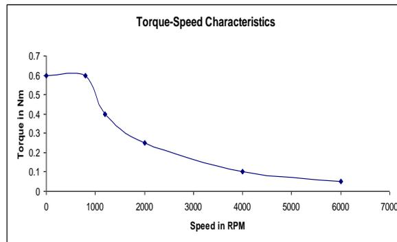
Fig: 8. Torque-Speed Characteristics of SRM.
