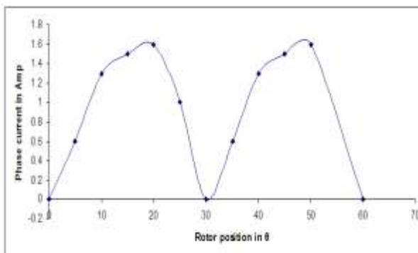
Fig: 7. Rotor Position-Phase current Analysis of SRM.
