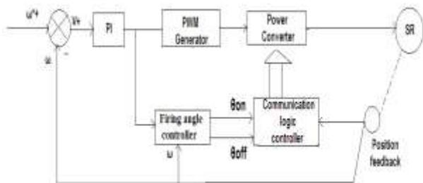
Fig: 6 Block diagram of current controlled Switched Reluctance drive
