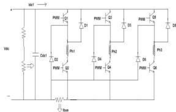
Fig: 5 Circuit diagram of proposed Voltage control drive
