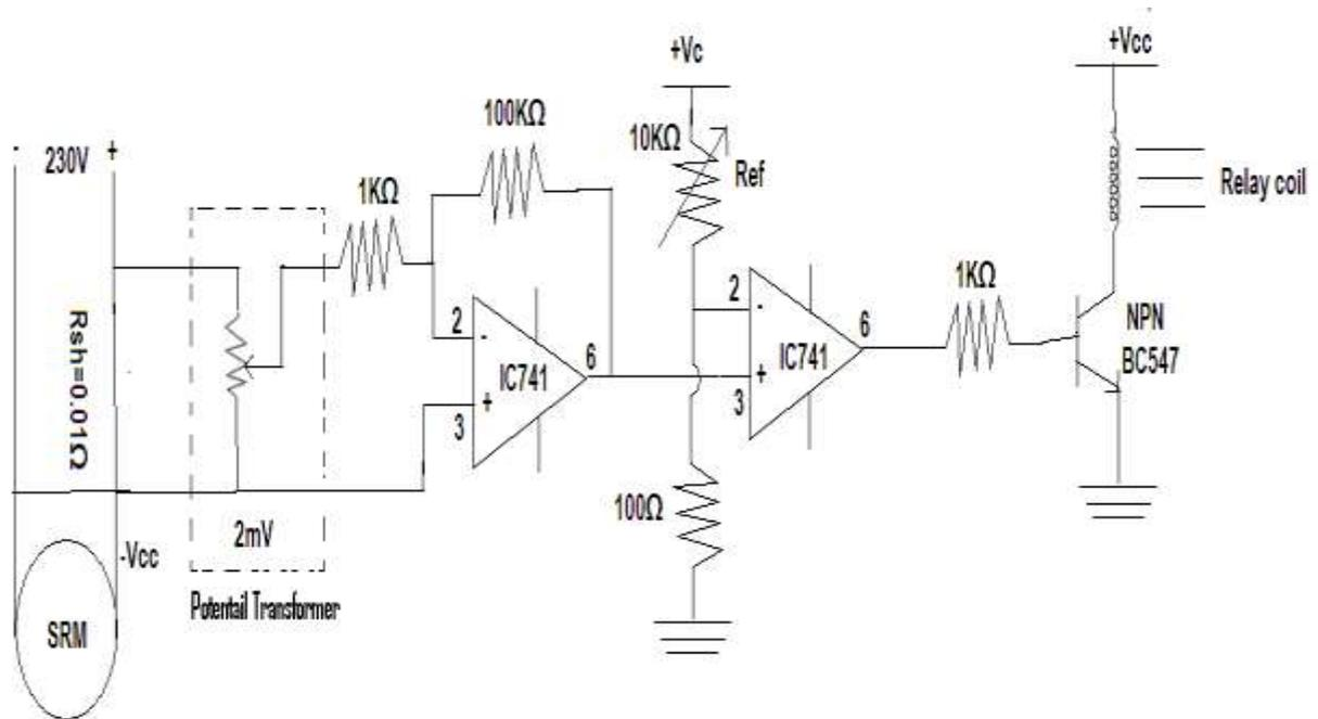
Fig. 1. Circuit diagram for conventional voltage control Method
