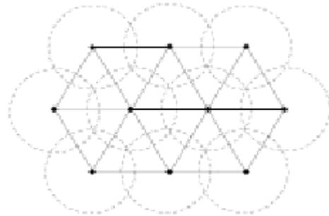
Fig "(b)": The structure of optimal coverage using the disk sensing model. This structure minimizes the overlap between the sensing ranges of nodes.
