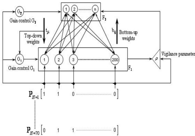
fig 2- Architecture of our ART1 neural network based clustered. The pattern Vector PH, which represents the access patterns of the host H is the input to the Comparison layer F1. The vigilance parameter determines the degree of mismatch that is to be tolerated. The nodes at the Recognition layer F2 represent the clusters formed. Once the network stabilizes, the top-down weights corresponding to each node in F2 represent the prototype vector for that node.
