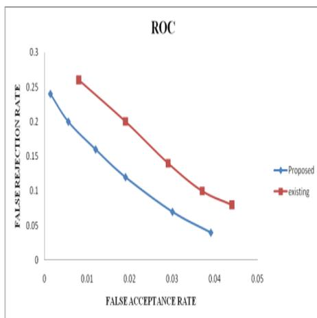
Figure 10: ROC GRAPH – Performance evaluation of Fingerprint Recognition for DB3\_A and DB4\_A with T=20
