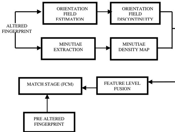
Figure 4: Flow Chart for Matching of Altered Fingerprint
